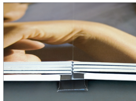
The flush-mount binding method created an elegant finish to premium books with single-print spreads.
